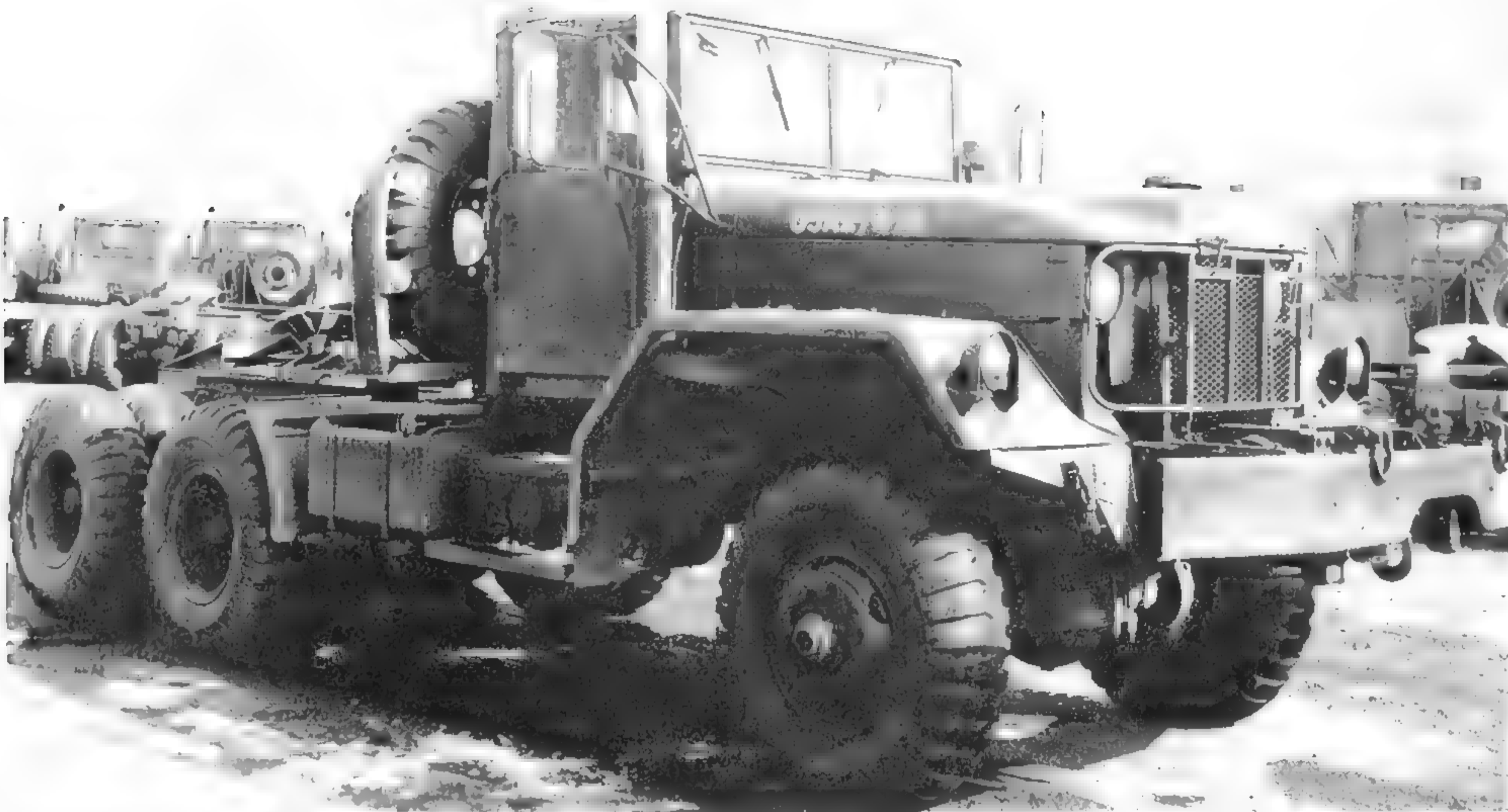
The M818 tractor, as well as the dump trucks, used a shorter wheelbase than the cargo trucks. (U.S. Army photo)
